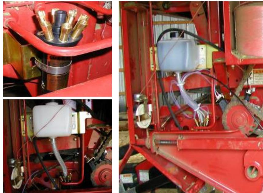
**Step 3** Cut the 5/8" ID hose as needed to connect the oil tank to the pump. Slide the hose clamps over each end of the hose and secure one end to the pump and one end to the tank.
