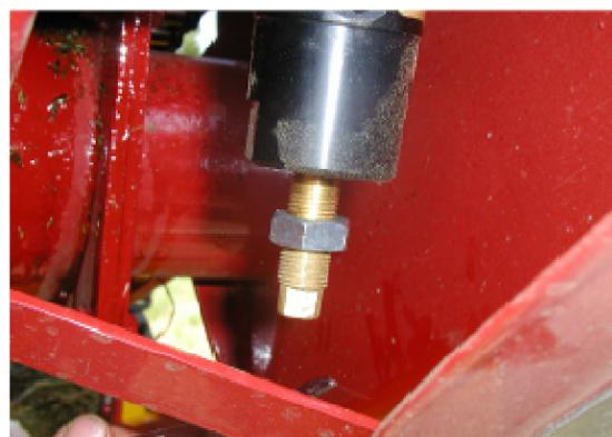
\*\*\*NOTE CNH SPECIFIES WE ONLY OIL 7 CHAINS ON THIS BALER. ONE CHAIN IS LOCATED BY A CLUTCH AND DOES NOT GET OIL\*\*\*
