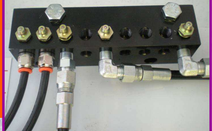
Grease Bank Manifold
