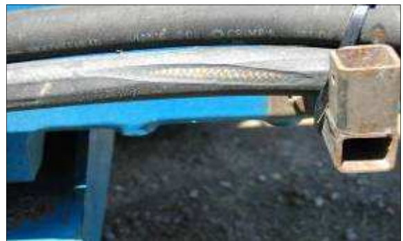
Protective sleeve would have likely saved this hose casing from being damaged
