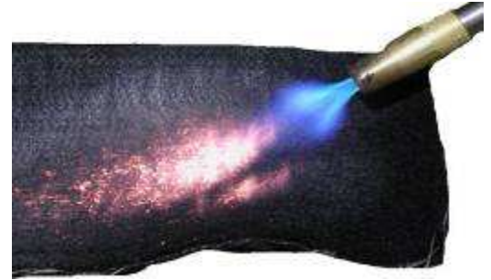
Carbon Fiber material resisting the open flame without any damage
