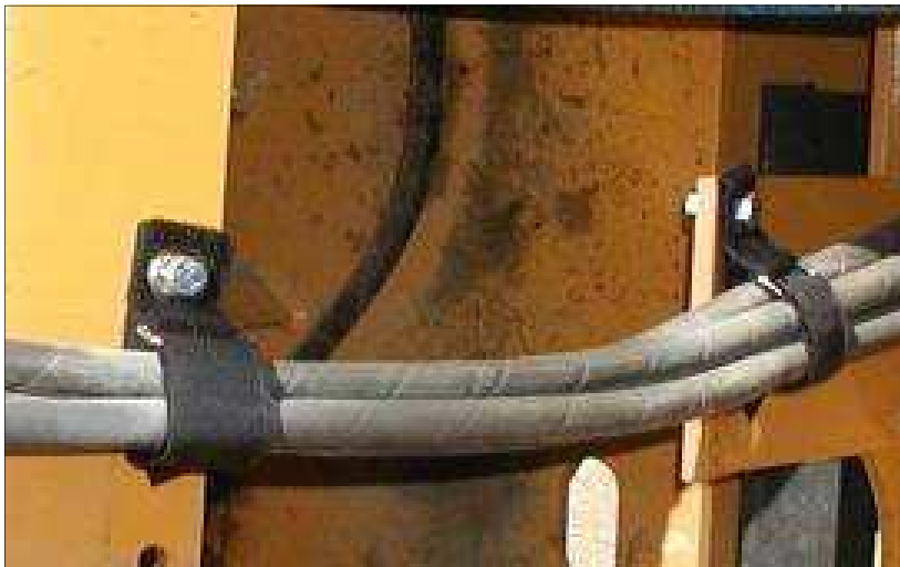
Heavy Duty Python Hanging Straps used to route hydraulic hoses
