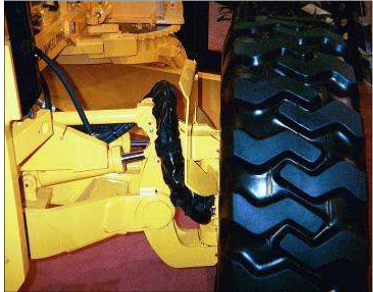
Above: Custom 5601 sleeve with heavy Urethane coating and straps prevent abrasion from steering components
