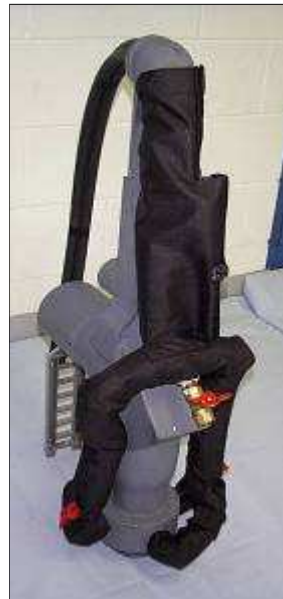
Special custom sleeve covers high temp tubes on a road patcher head preventing against operator injury
