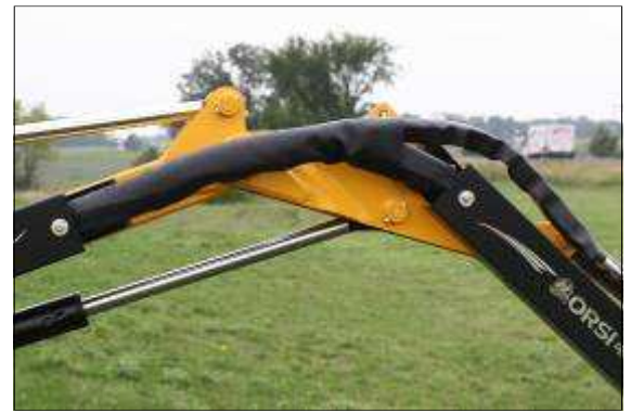
Pinch point protection
