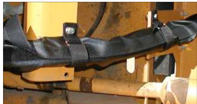
Sidewinder Sleeve is easily applied with Hanging Strap to contain and protect the hoses
