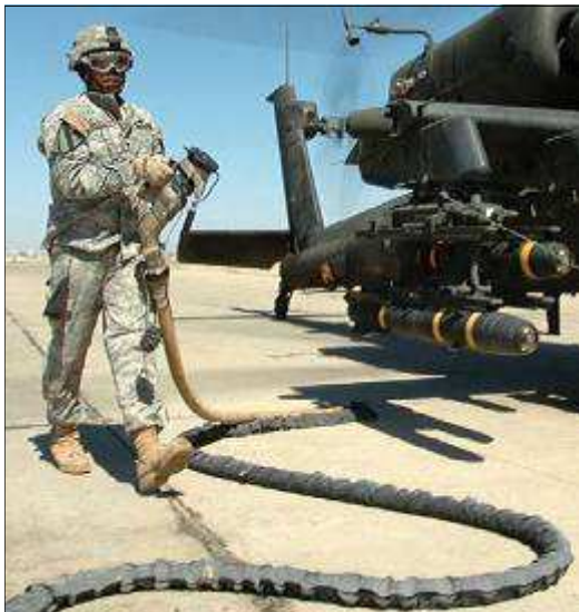
HOT refueling application for military helicopter. Sidewinder Sleeve is wrapped around refueling line to protect expensive refueling line from abrasion.
