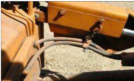
Over time, fixed clamps may damage the hose.
