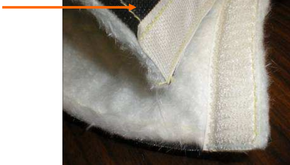
Close-up of sleeve with insulation and high temperature hook and loop closure
