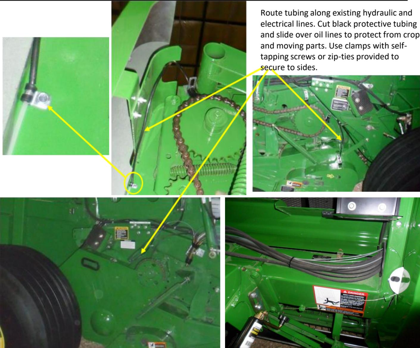
Route tubing along existing hydraulic and electrical lines. Cut black protective tubing and slide over oil lines to protect from crop and moving parts. Use clamps with self-tapping screws or zip-ties provided to secure to sides.
