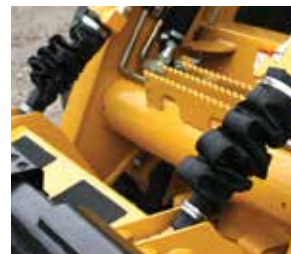
Hydraulic cylinders rely on the flexibility of 5601 to prevent contamination to piston rods.
