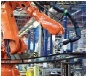
Robotics applications need 18411 to bundle & protect articulating hoses.
