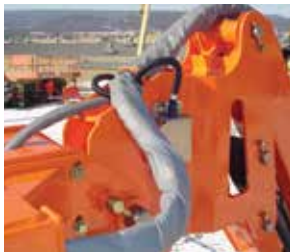
Protects hoses from welding and grinding spall in shipbuilding applications.
