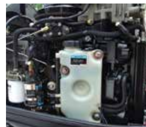
Outboard marine engines shield electrical wiring from high heat engine exhaust.
