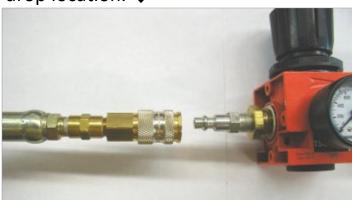
Connect the air tool used most often at the air drop location.
