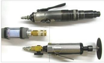
It is important to note that most air tools have 2 CFM ratings: Under no load (free moving) and Under load (doing work)
